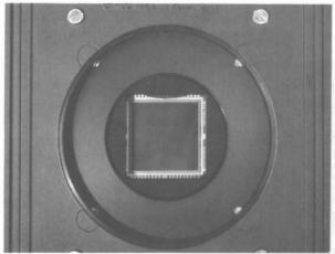
Figure 3 CCD sensor of the eyelike camera
