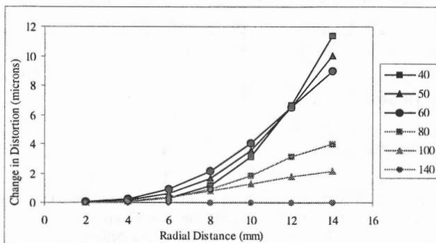
Figure 3. Change in the radial lens distortion profiles with magnification for the DCS460 with the 20mm lens.
