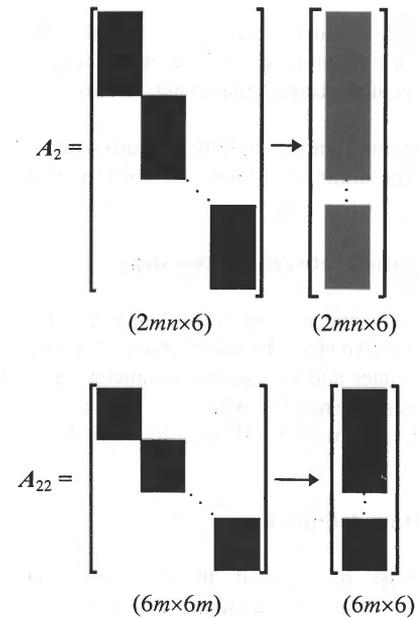
Figure 4-3 The structures of the matrices  $A_2$  and  $A_{22}$
