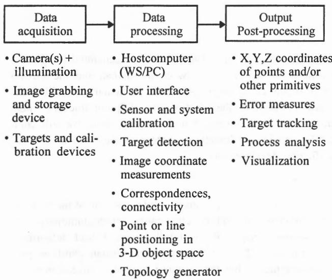
Figure 1: Components of a videogrammetric system
