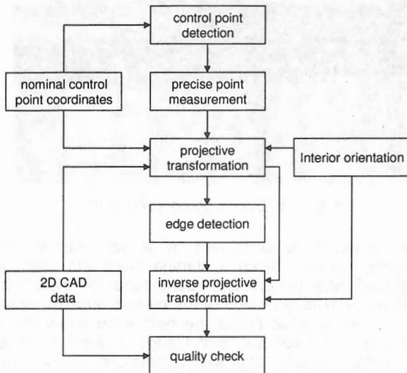
Figure 10: Measurement process
