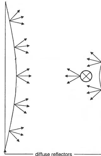
Figure 3: Diffuse illumination technique
