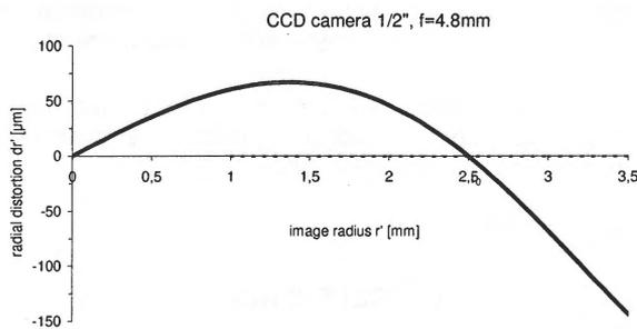
Figure 7: Radial distortion
