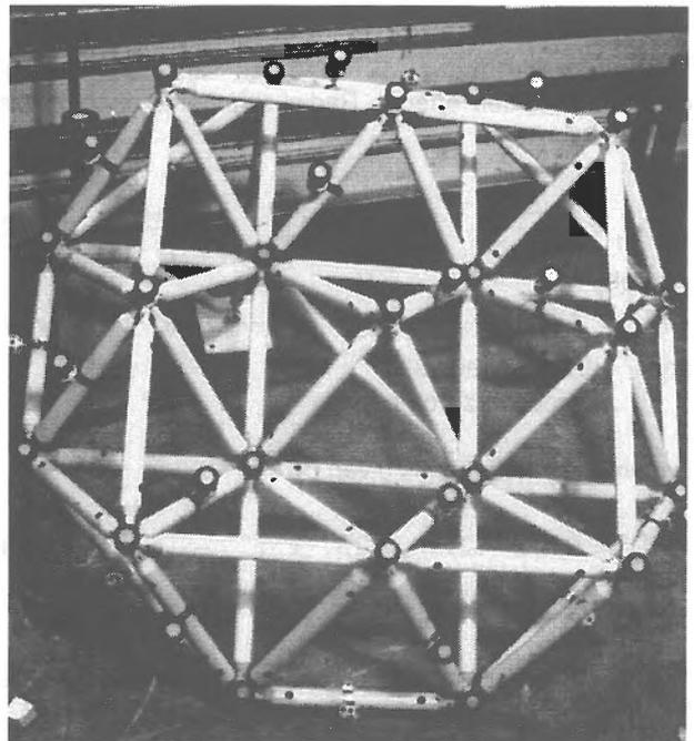
Figure 4: Testfield with control points
