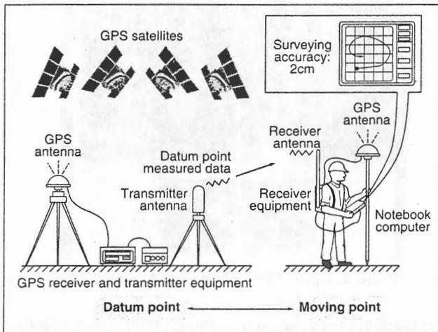
**Figure 1.** The GPS navigation-type surveying system
