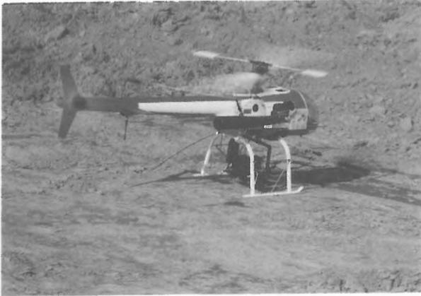
**Photo 3.** Photographing from Radio control helicopter
