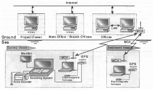
Figure 2 Configuration Diagram of the System
