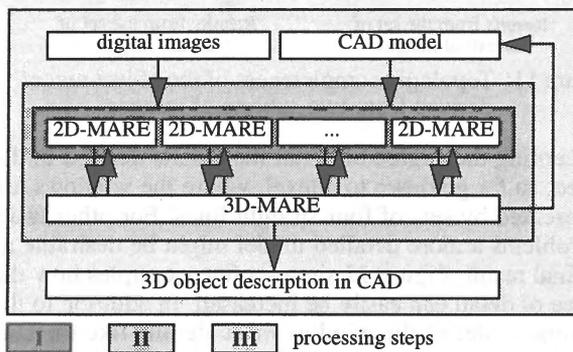
Figure 8: Processing steps in DIPAD (MARE = automatic measurement of architectural elements)
