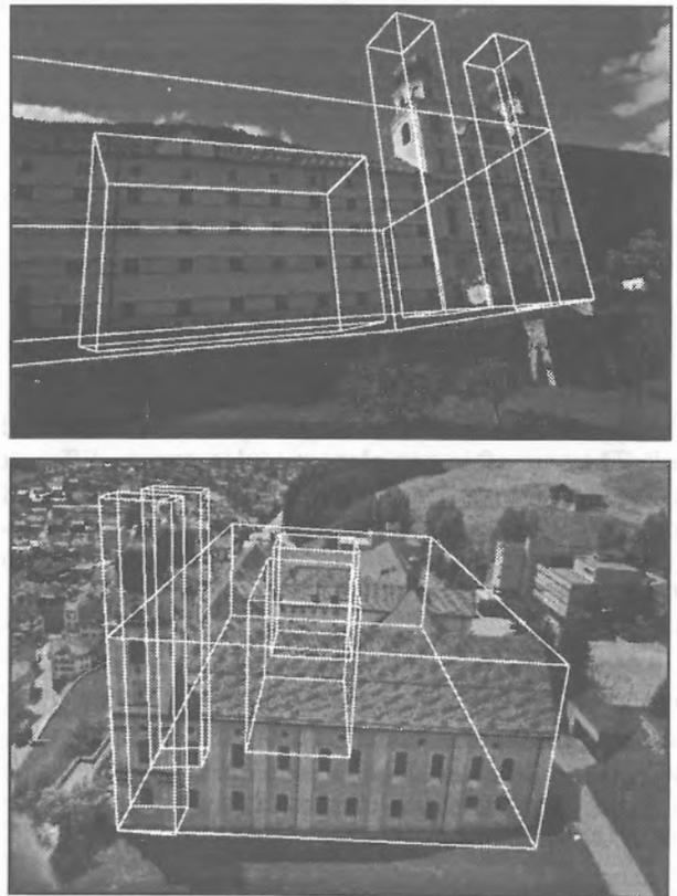
Figure 7: Two examples for the projection of the initial model into acquired images
