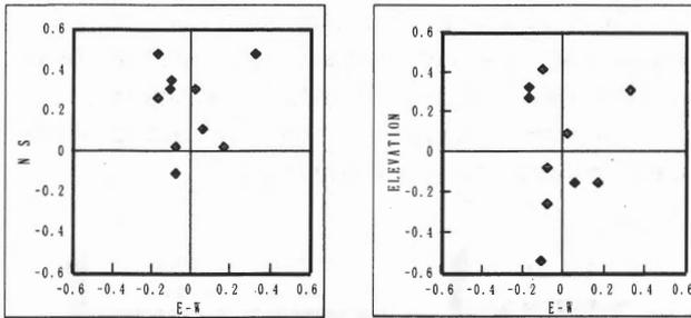
Fig 3. Relative errors of airborne laser survey ( m )
