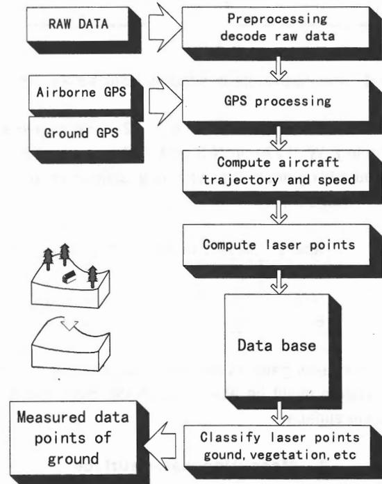
Fig.2 Logical sequence of post-processing
