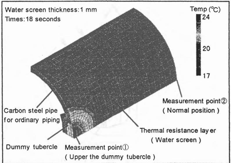
**Fig.3 Simulation result of temperature distribution at the water screen surface**
