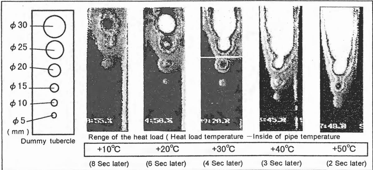
**Fig.7 Example of the examination results of a range of the heat load given to the thermal resistance layer**
