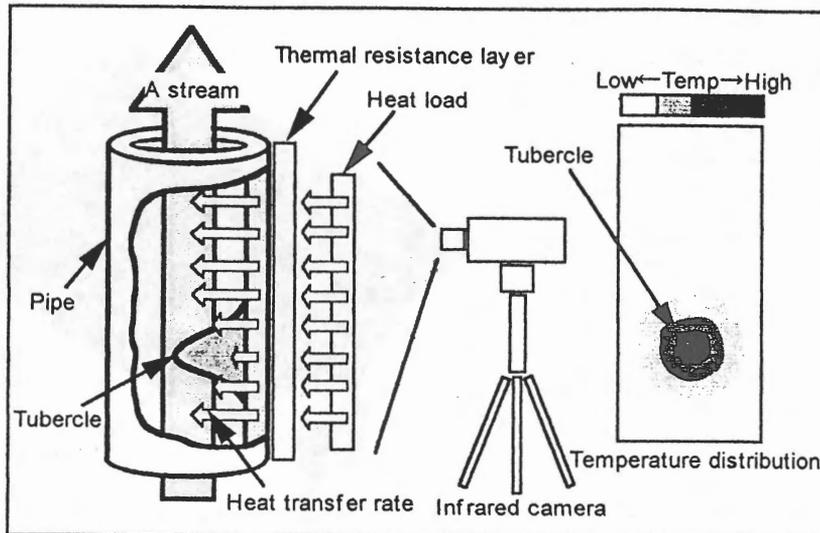
Fig.1 Diagnose the pipe with the use of infrared camera
