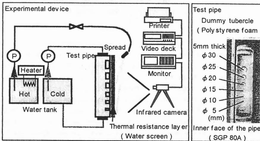
Fig.2 Experimental device and a test pipe
