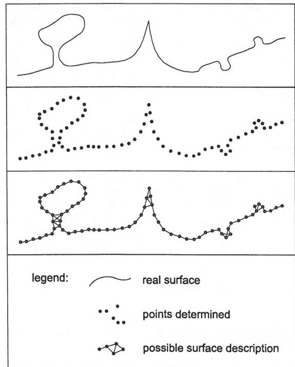
Figure 2: Correctness of the TIN in dependence on the surface shape
