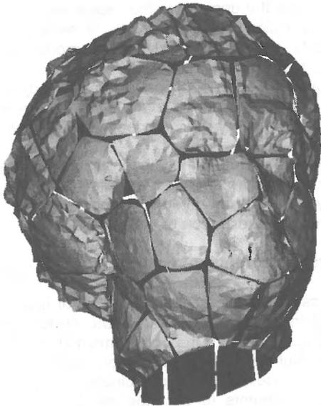
Figure 1: Division of a surface into individual processed parts
