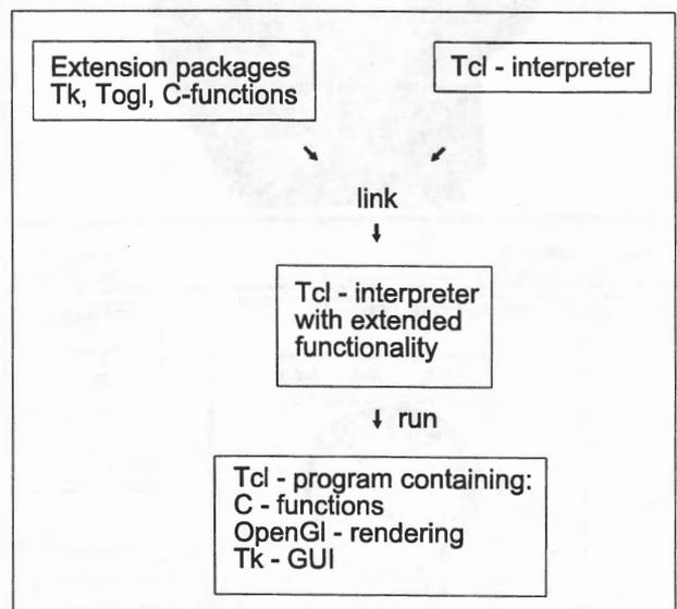
Figure 7: Linkage and execution of the visualization program
