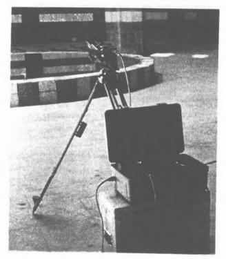
Fig.-1 Cavity Monitoring System
