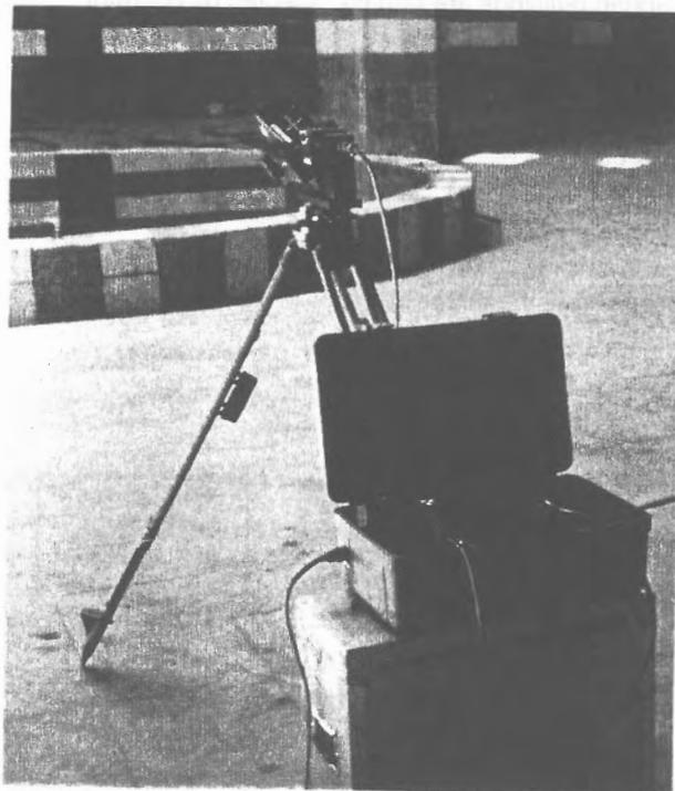
Fig.-1 Cavity Monitoring System
