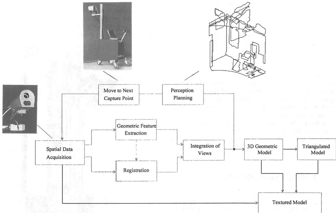
Figure 1: Paradigm for Photo-Realistic 3D Scene Reconstruction.
