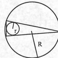
Figure 5: Triangle aspect ratio.
