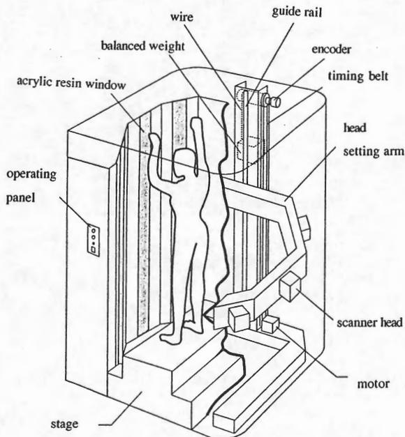
Fig.7 Structure of BL scanner
