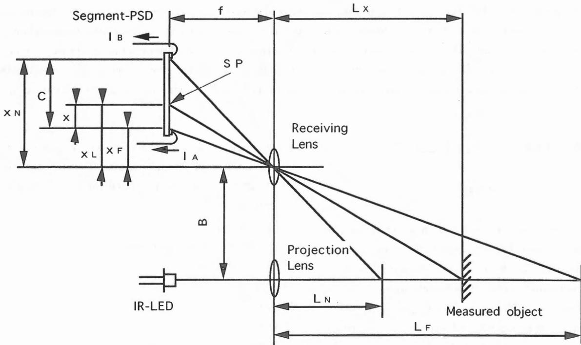
Fig.1 Optical system for distance detection
