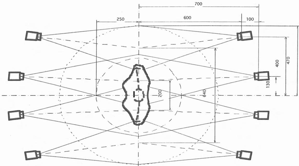
Fig. 6 The arrangement of the Scanner Head
