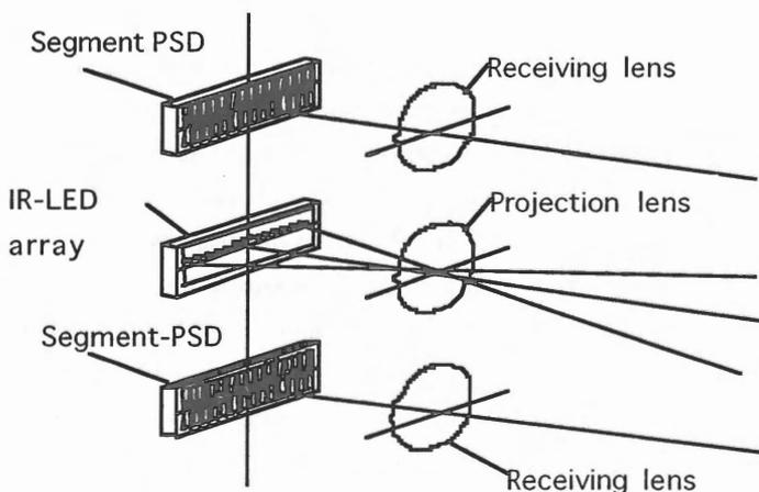
Fig.5 Optical system for scanner head
