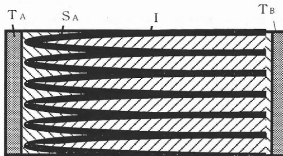
Fig. 3 Pattern structure of segment PSD
