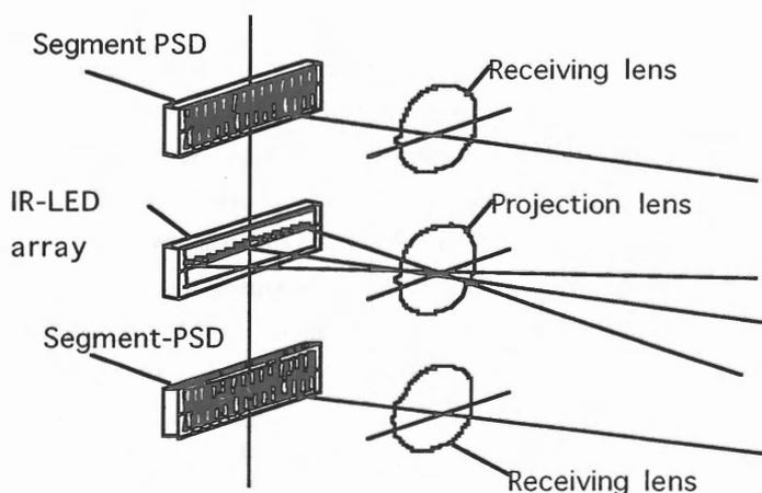
Fig.5 Optical system for scanner head
