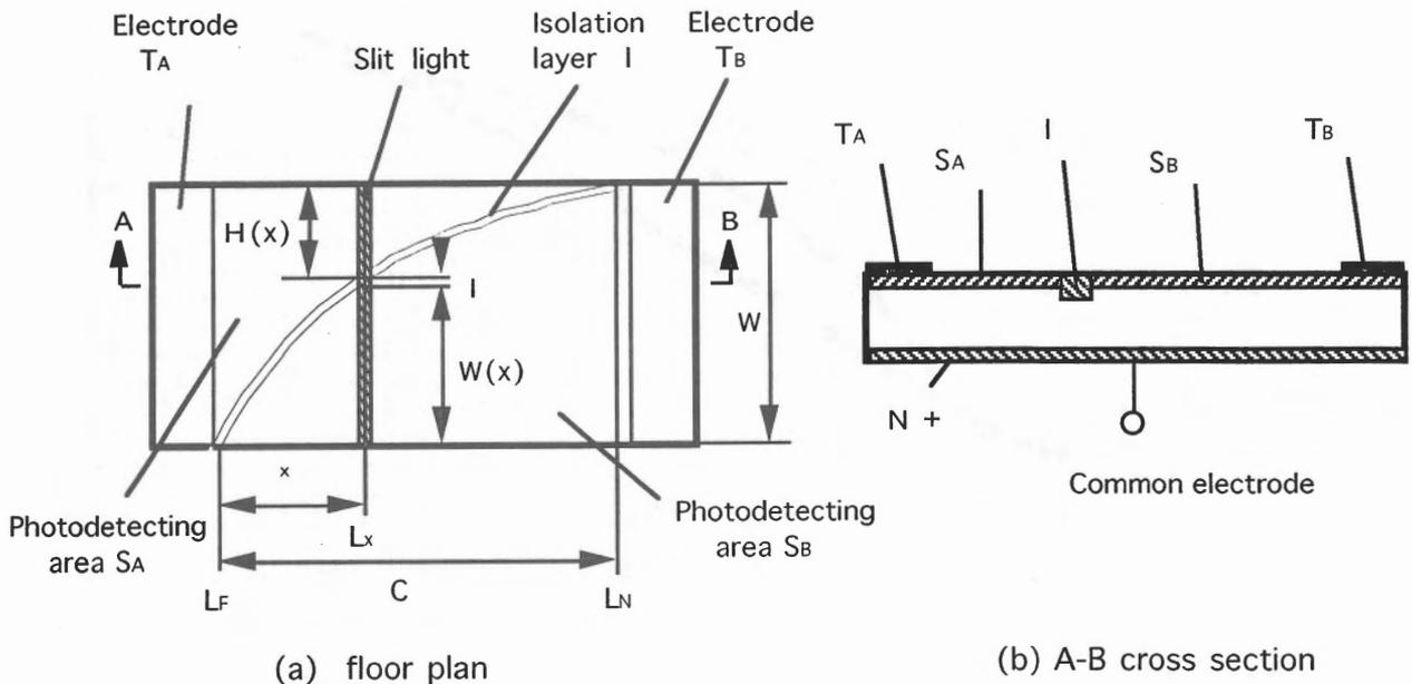
Fig.2. Structure of Segment-PSD
