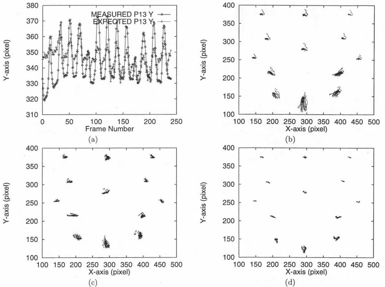
Figure 6: (a) Vertical motion of the point C2. Cross: estimation. Diamond: true position. The amplitude of the expected vertical motion is smaller than actual motion. This is probably caused by insufficient span of the basis. Figures (b)-(d) are the trajectories of markers. Figure (b) is the output of tracker (actual motion). Figure (c) is the estimated trajectory for the training sample, and (d) is the result for a test image.
