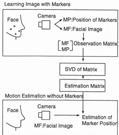
Figure 3: Block-diagram of the process. In the first learning stage, an image vector  $f_i$  of the face is measured with the positions  $p_i$  of markers. For the sequence  $\{i = 1, \dots, n\}$ , singular value decomposition is applied. Using the result the algorithm estimates *virtual marker position* only from  $f$ .
