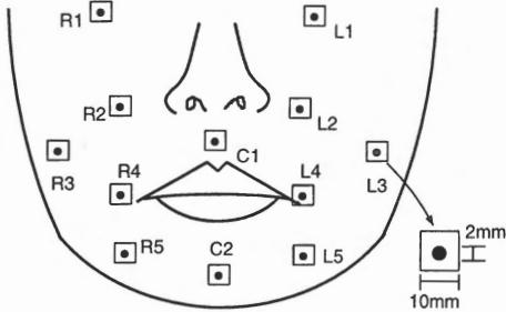
Figure 1: First stage observes a facial image sequence with markers. The trace  $P$  of the markers are measured by a tracking program. In our experiment thirteen points are located around lips. A marker is a white square ( $10\text{mm} \times 10\text{mm}$ ) sticker in the center of which a black circle ( $2\text{mm}$ ) is printed.
