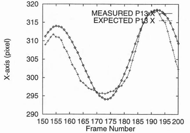
Figure 5: An example of estimation. Frames from 0 to 149 are the learning sample. The position of the markers are estimated from  $f$  for 150-200 frames. Crosses: estimation. Diamonds: true position.
