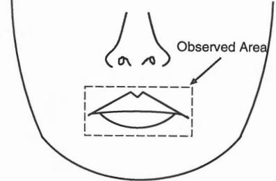
Figure 2: A vector  $f$  of gray level values are measured within the area indicated as a square. For reduction of computational cost, the pixel size of the image is re-quantized by 1:4.
