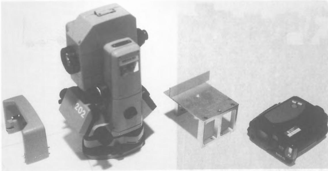
Figure 1 - Total Station, Adapter and Digital Camera
