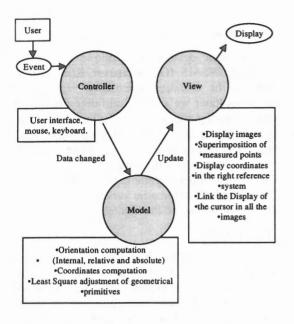
Figure 2. MVC synoptic scheme in Arpenteur.
