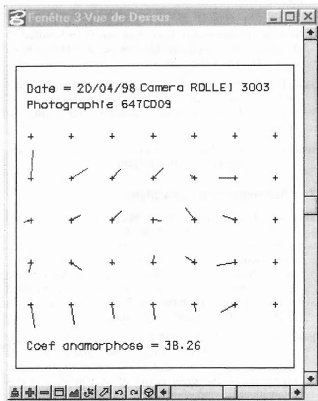
Figure 5. Automatic report of reseau deformations in MicroStation file format
