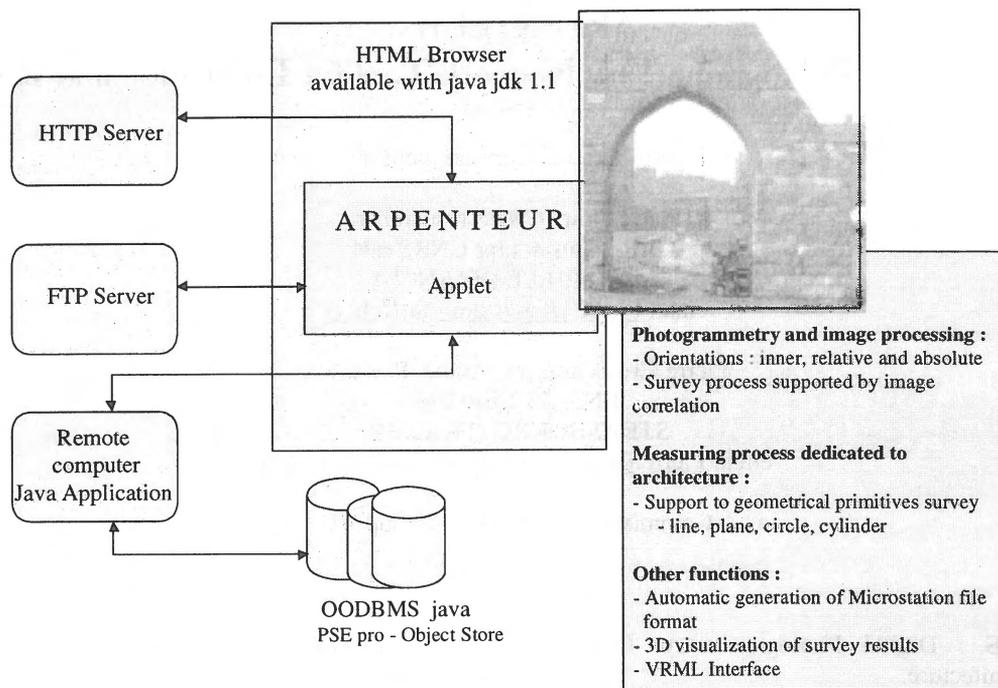
Figure 1. ARPENTEUR's project synoptic scheme.
