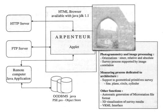
Figure 1. ARPENTEUR's project synoptic scheme.
