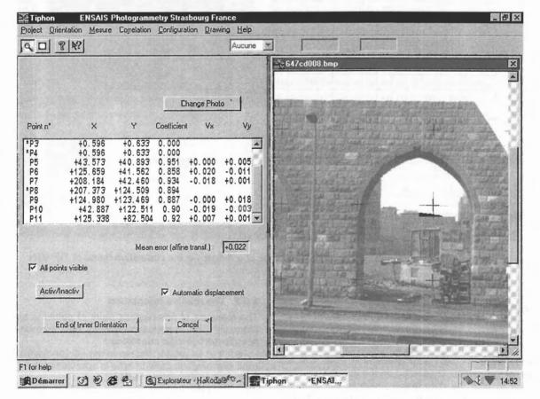
Figure 3 : the dialogue box of the inner orientation with TIPHON
