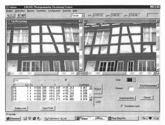
Figure 10 : digital stereoplotting (FUJIX DS-300 images) of a typical Alsacian House in the "Petite France" area at Strasbourg.
