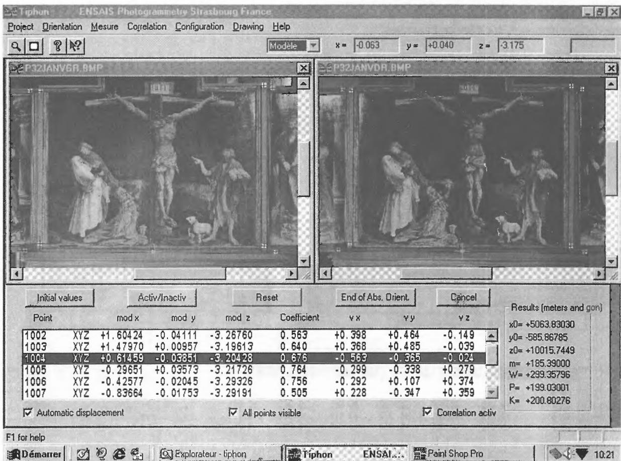
Figure 7 : the absolute orientation (here a spatial similarity transformation) with TIPHON
