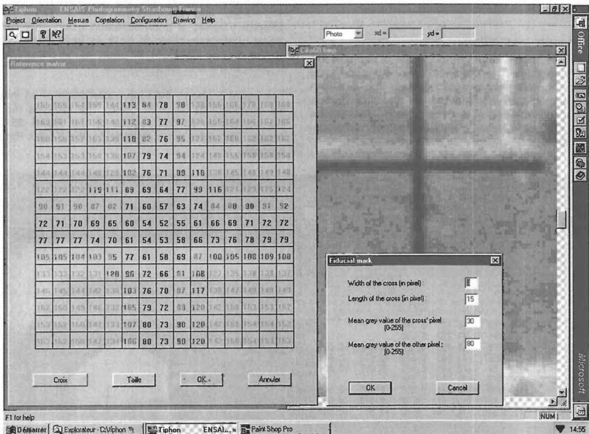
Figure 2 : definition of the target matrix (here a cross of a reseau) in the correlation menu of TIPHON
