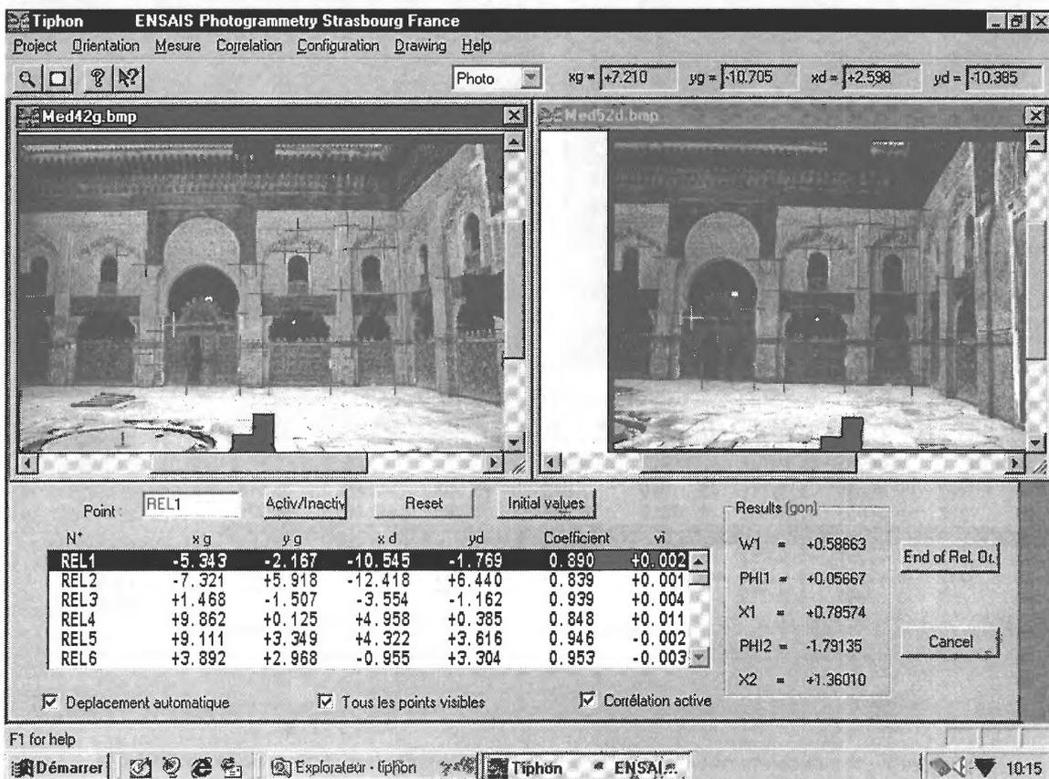
Figure 5 : the relative orientation with TIPHON.
