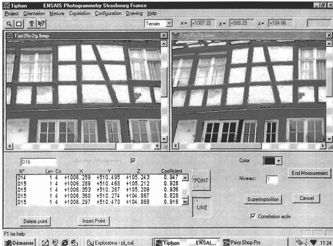
Figure 10 : digital stereoplottting (FUJIX DS-300 images) of a typical Alsacian House in the "Petite France" area at Strasbourg.
