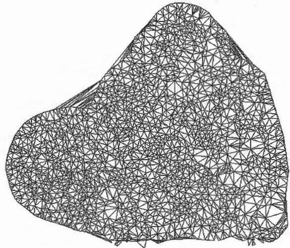
Figure 13. Generated Delaunay triangular mesh of Fig.12(a).
