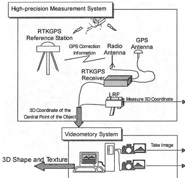
Fig.8 3D Coordinates Measurement System
