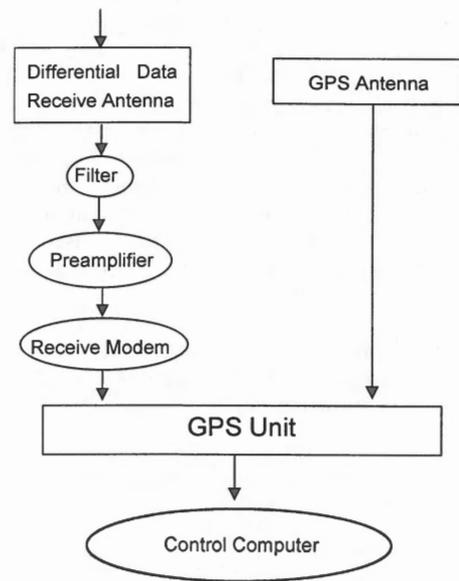
Fig.5 Processes at a remote receiver system
