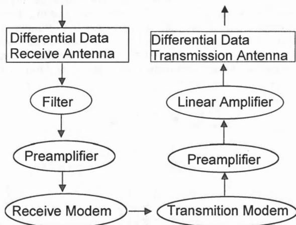
Fig.4 Processes at the relay station
