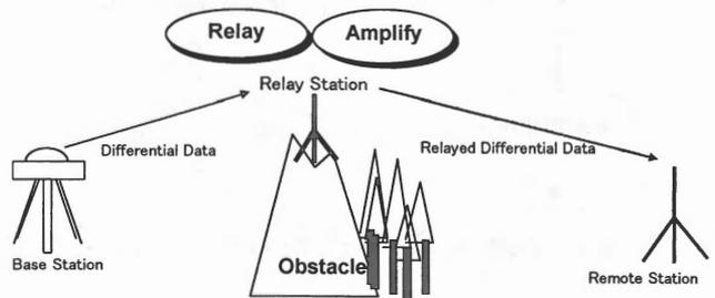
Fig.2 RDGPS system with a relay station
