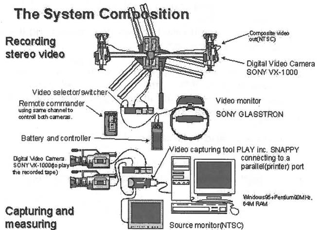
Fig.9 The system configuration of videometry
