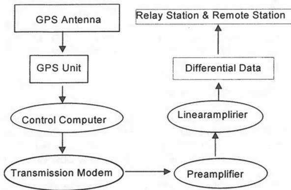
Fig.3 Processes at the base station system
