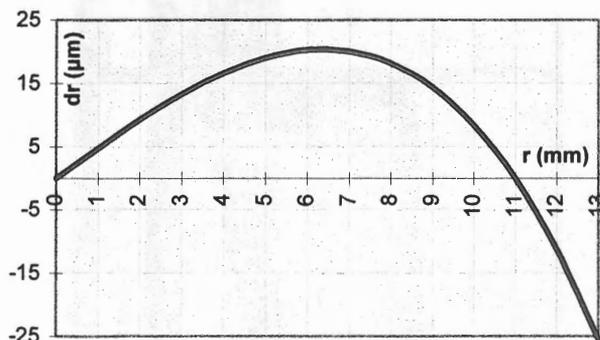
Figure 5: Radial distortion curve for Kodak DCS420
