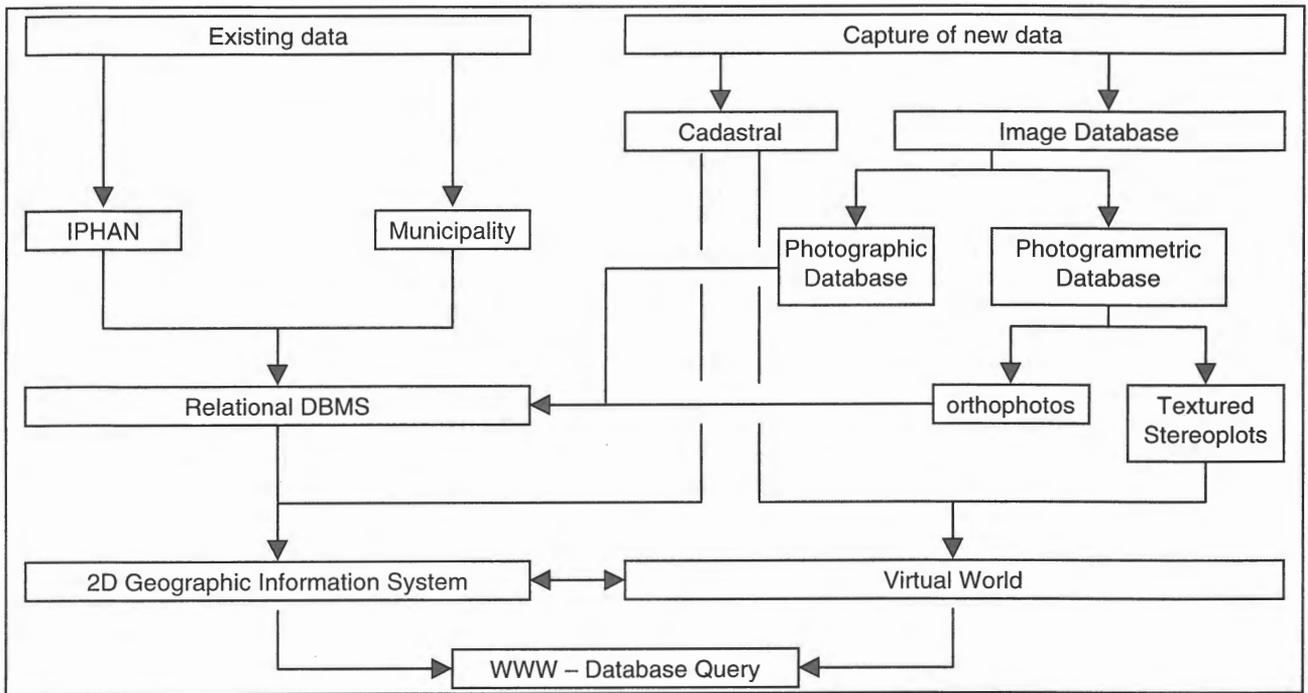
Figure 1 – Flowchart showing the construction of the 2D and 3D Information Systems.
