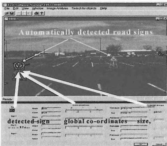
Figure 2. The road sign - automatically recognised and positioned (in a global frame).
