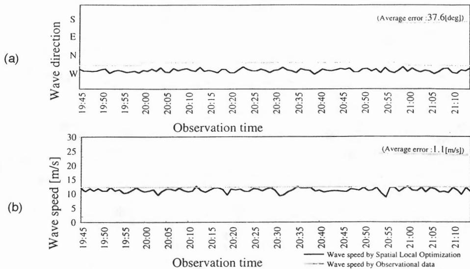
Fig.9 Result of time series of wave direction and wave speed by SLO
