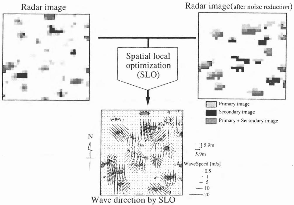
Fig.4 Flow diagram showing SLO method using radar image
