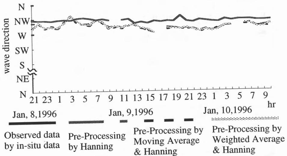
Fig.7 The result of comparison between wave direction by FFT r and in situ data
