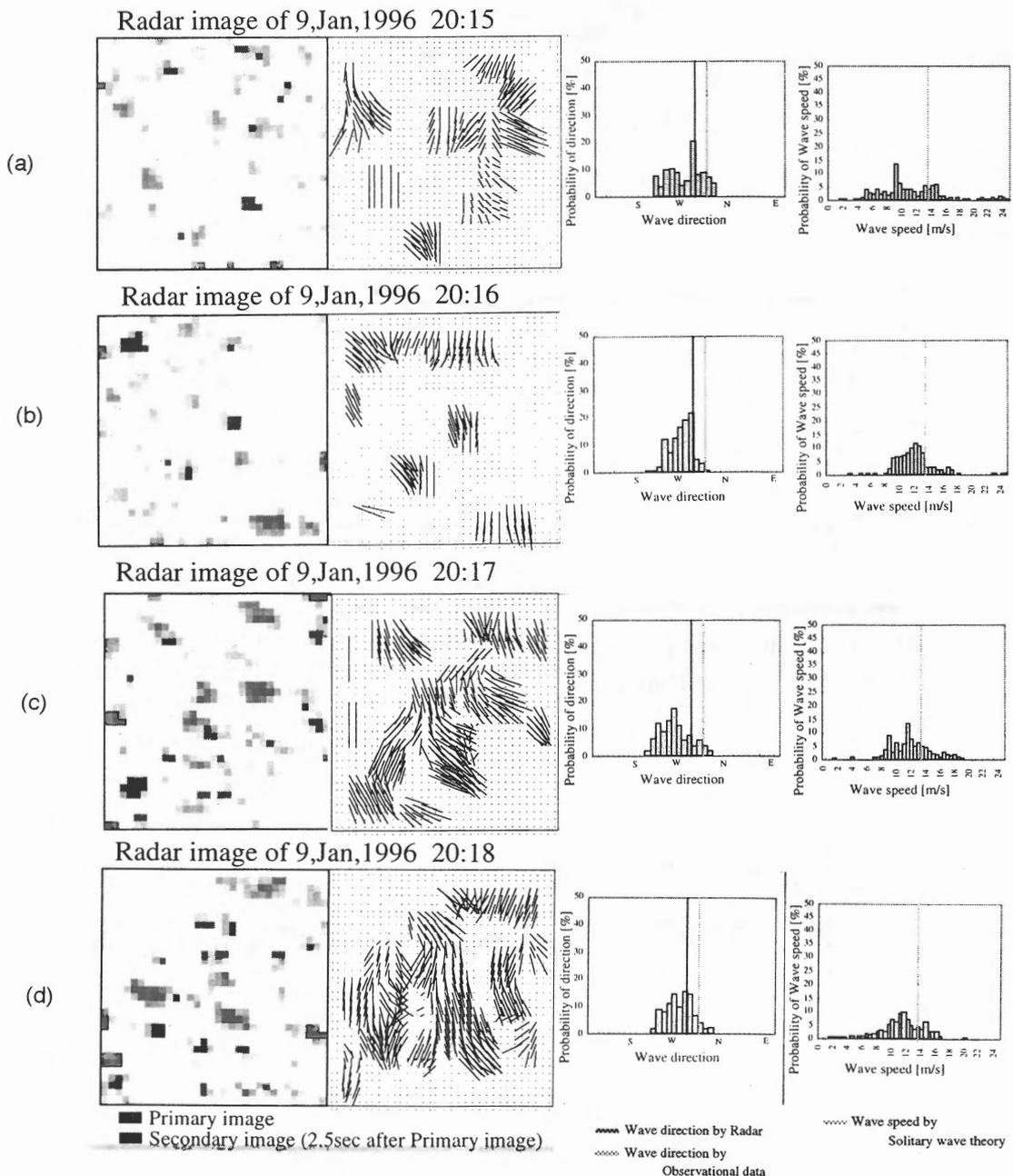
Fig.10 2-D field of wave direction and wave speed by SLO
