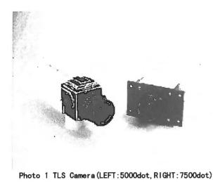
photograph, a digital data recorder and controller. And to analysis the acquired data which flew the sky of the highway of the measuring, the speed of the vehicles can be measured. The principle of measurement velocity of vehicle form digital image by TLS system s mentioned below.
