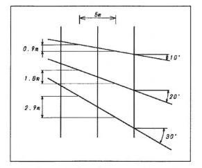
Figure 7 The deviation of the position by the angle of the road and the line
