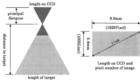
Figure 3. target length and principal distance
