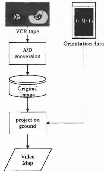
Figure 6. making process
