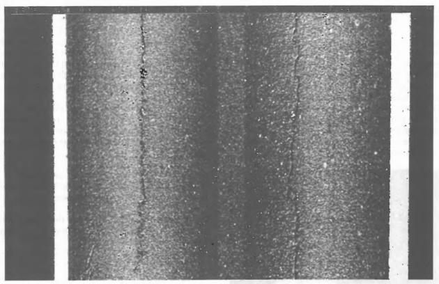
Fig.5. Crack image (Vertical direction)
