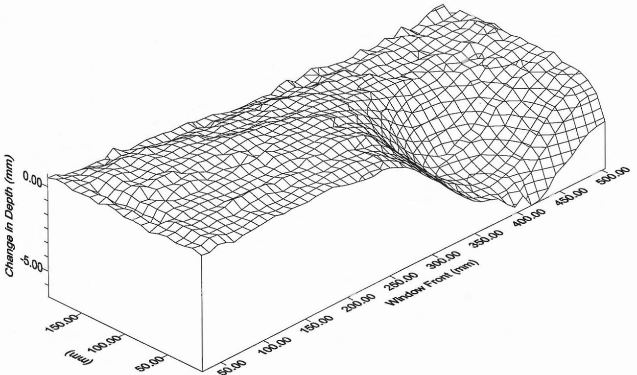
Figure 5. Difference between the original soil surface and that computed after collapse.
