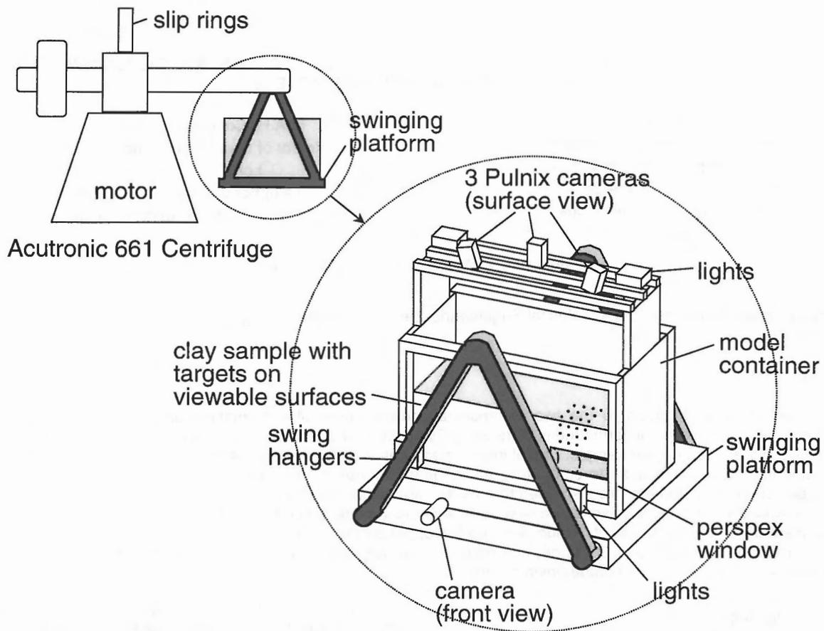
Figure 1. The arrangement of the geotechnical centrifuge, detailing the camera configuration used.
