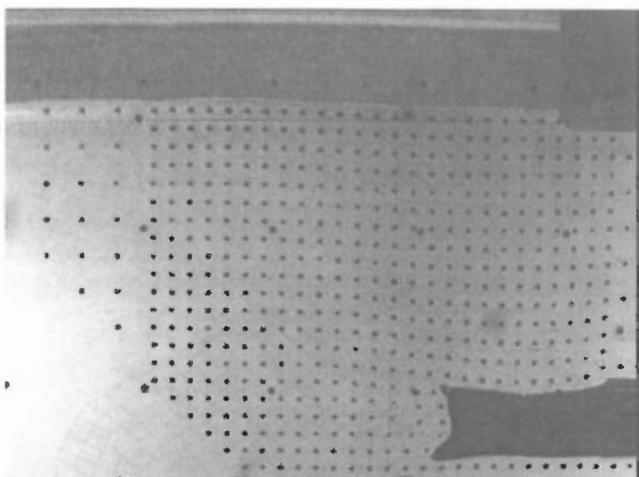
Figure 2. Soil model front view showing a tunnel section during collapse.
