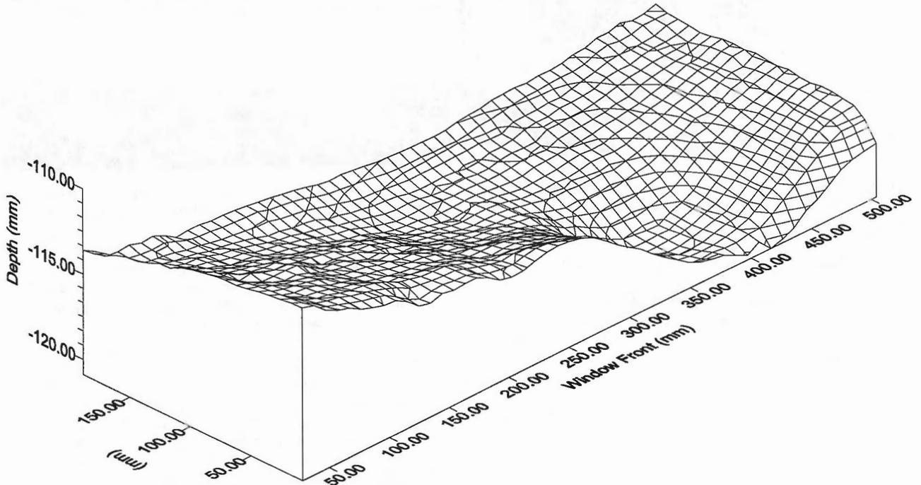
Figure 4. Soil surface computed after collapse.
