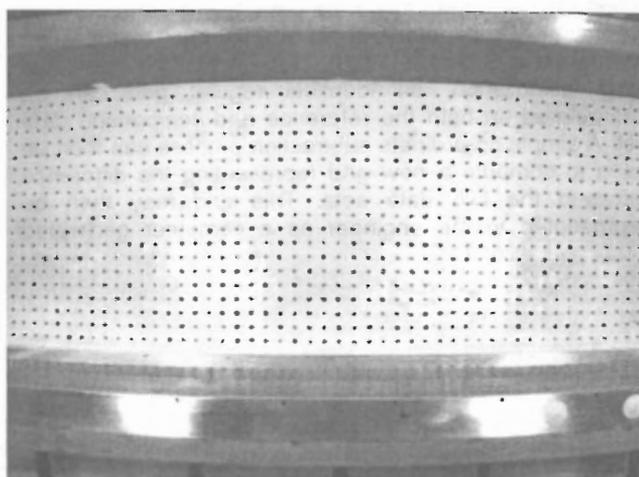
Figure 3. View from the central camera (of three) monitoring targets on the soil surface.
