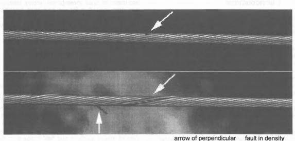
arrow of perpendicular fault in density arrow of diagonal fault in shape Figure 9. detection example
