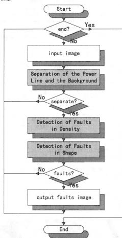
Figure 7. detection of faults flow
