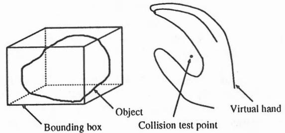
Figure 10. Collision detection method.
