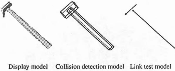
Figure 8. Three models prepared for a hammer.
