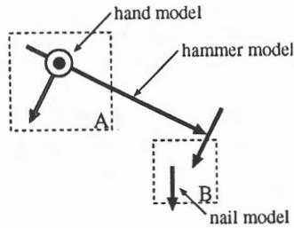
Figure 13. Relation among hammer used as extractor, hand and nail.
