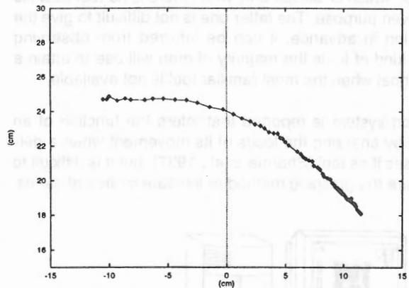
Figure 7. A locus of a hammer head used as puller.
