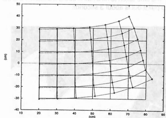
Figure 3. Distortion of magnetic field.
