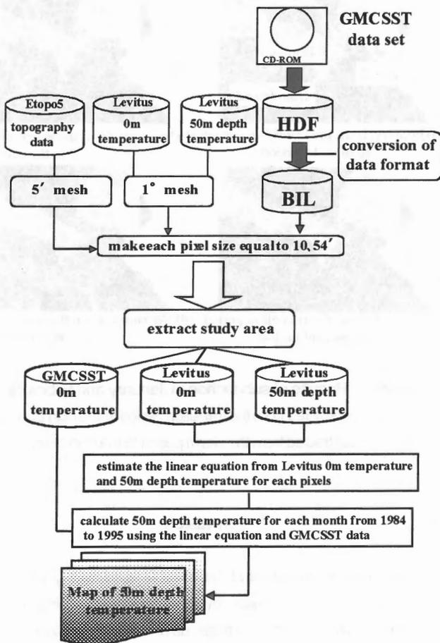
Figure 4 Flow Chart of data processing and method of calculating the temperature at the 50m depth
