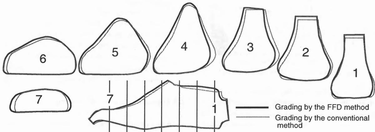
Figure 8 Application for shoe last grading
