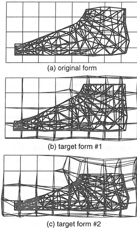
Figure 3 Movements of control lattice points
