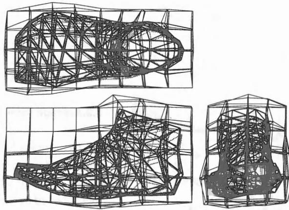
Figure 7 Movements of control lattice points to convert from a foot of E width to a foot of 4E width
