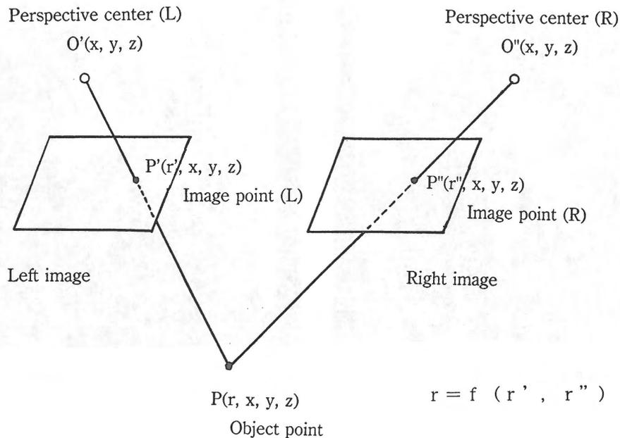
Figure 1 The method for making an ortho-image using stereoscopic images
