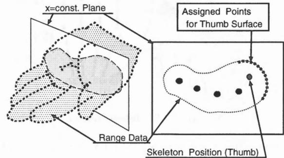
Figure 4. Procedure to get the polygon vertices
