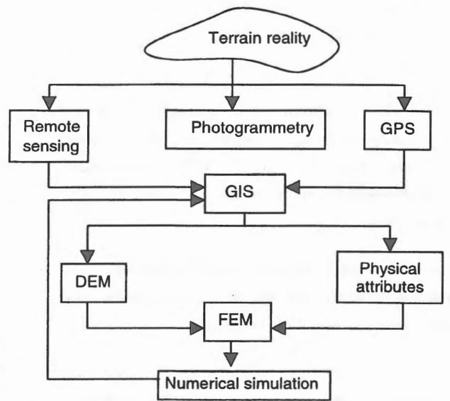
**Figure 2** Linkage between GIS and FEM
