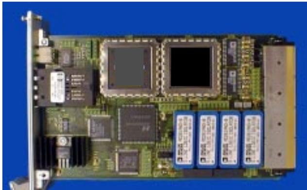
Figure 6. PCB of the Signal Processing Module
