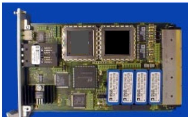
Figure 6. PCB of the Signal Processing Module
