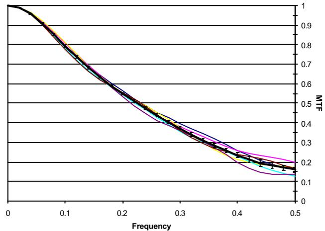
Figure 6 On orbit measured system MTF (exclusive of display)
