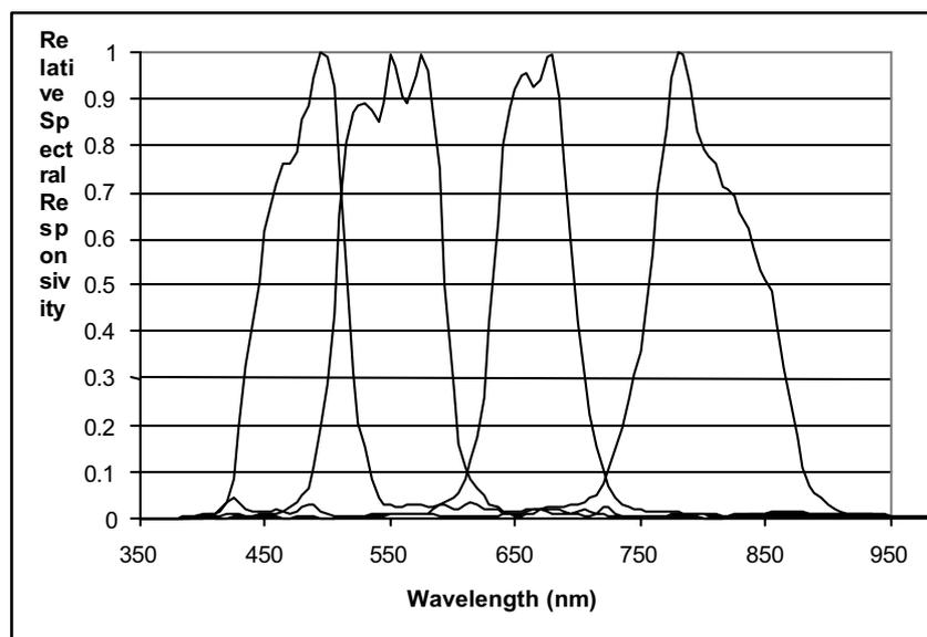
Figure 4 Normalized multispectral filter response
