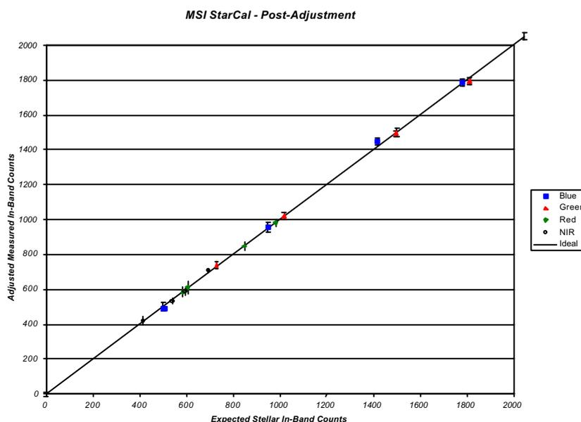
Figure 8 Multispectral calibration from star data
