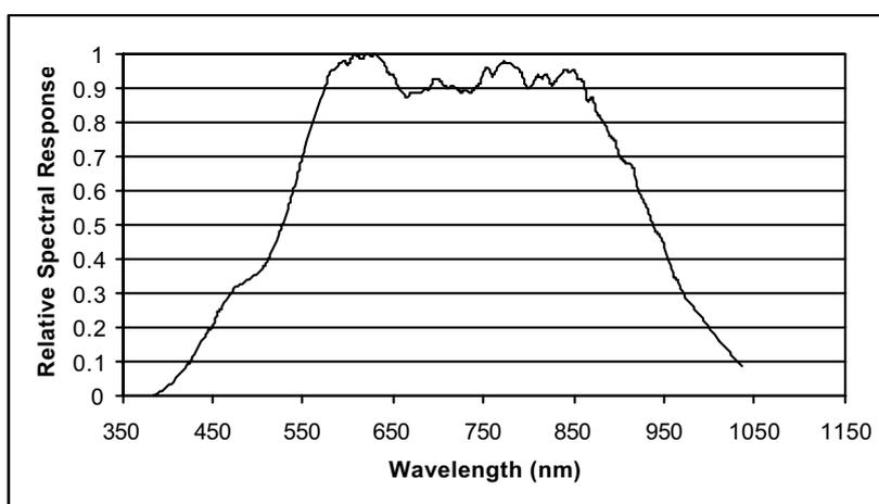
Figure 2 Pan CCD relative spectral response
