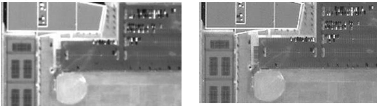
Figure 7 IKONOS one meter image without and with MTFC
