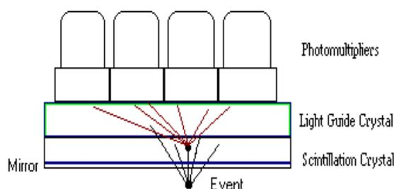
Figure 1. Photomultiplier Based Scintillation Sensor
