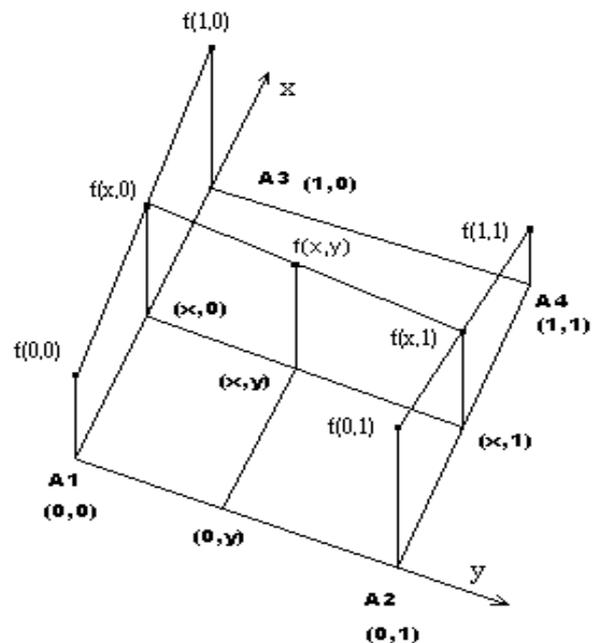
Figure 3, 2-D Bilinear Interpolation
