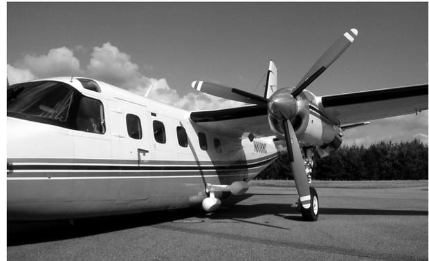
Figure 1: Gulfstream Commander 1000 with AeS-1 X-band antenna boom construction
