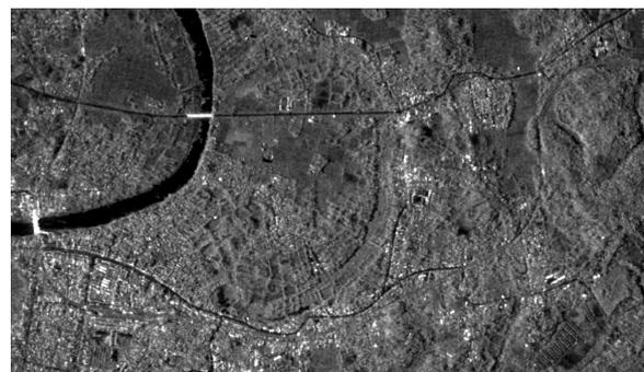
Figure 4: SAR ortho image, Indonesia, spatial resolution 2.5 m x 2.5 m
