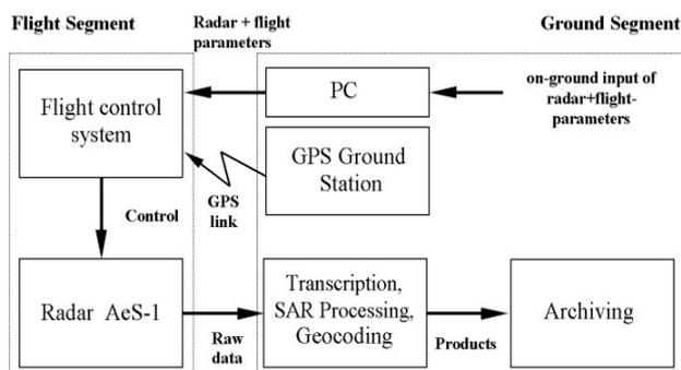
Figure 3: Block diagram of the AeS-1 system
