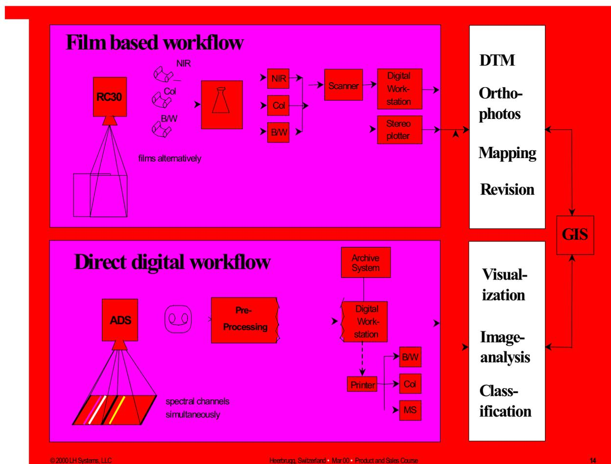
Figure 3: Film based and direct digital workflow
