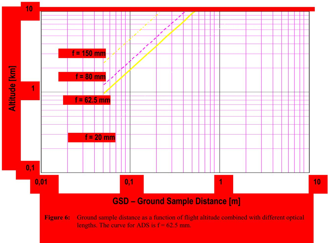
Figure 6: Ground sample distance as a function of flight altitude combined with different optical lengths. The curve for ADS is  $f = 62.5$  mm.
