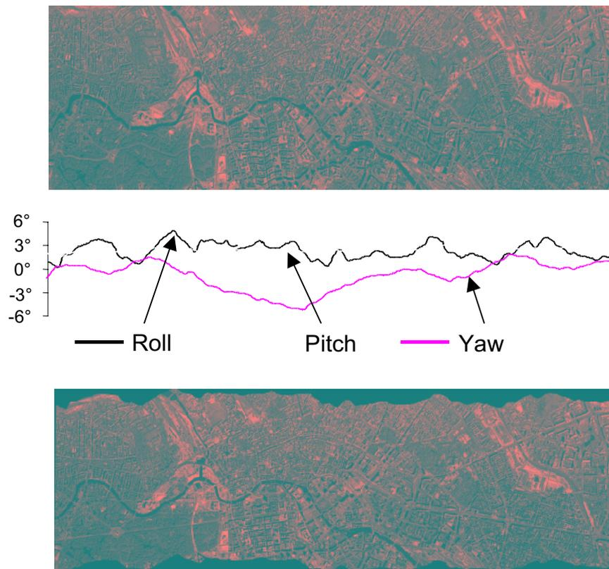
**Figure 4:** Imagery over Berlin with a 3 line scanner
