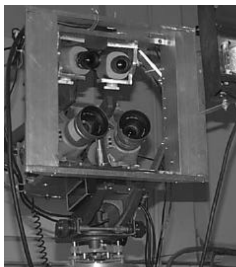
Figure 3: The mount holding the multiple cameras system in its first configuration (4 cameras).
