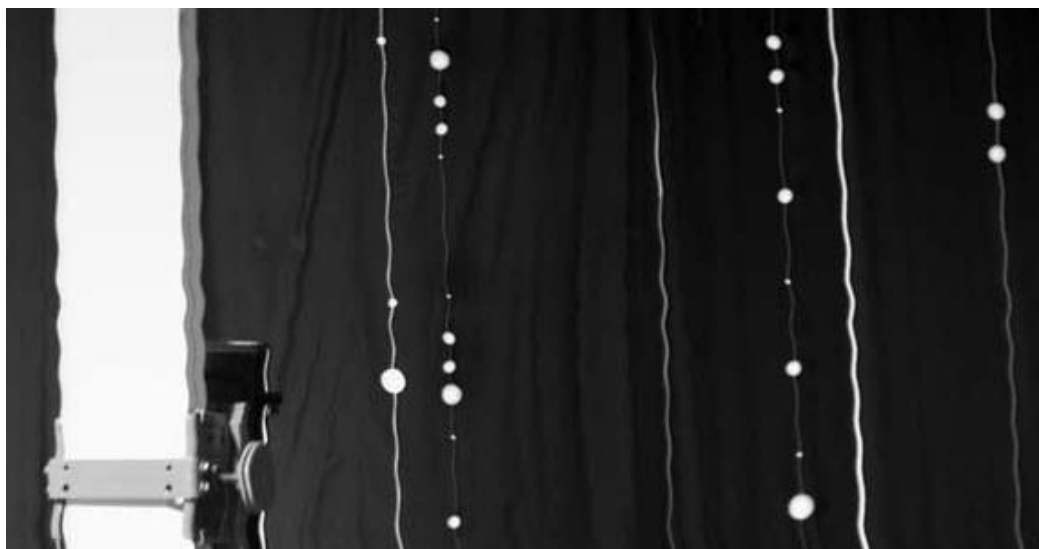
Figure 4: An example of an image distorted by a jitter of about 3 to 4 pixels
