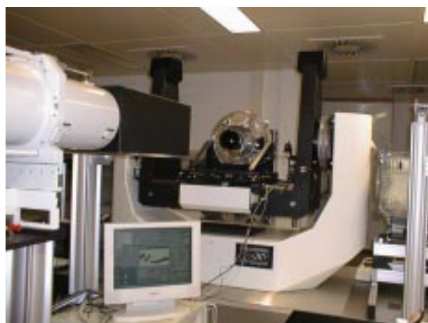
Figure 4. The engineering model of the ADS40 during the calibration procedure
