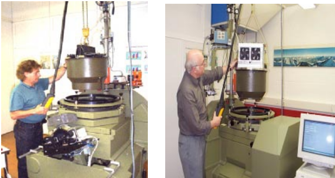
Figure 9. Inserting optical systems into the CVG: a) objective UAGS for testing the optics b) engineering model of the ADS40 for calibration
