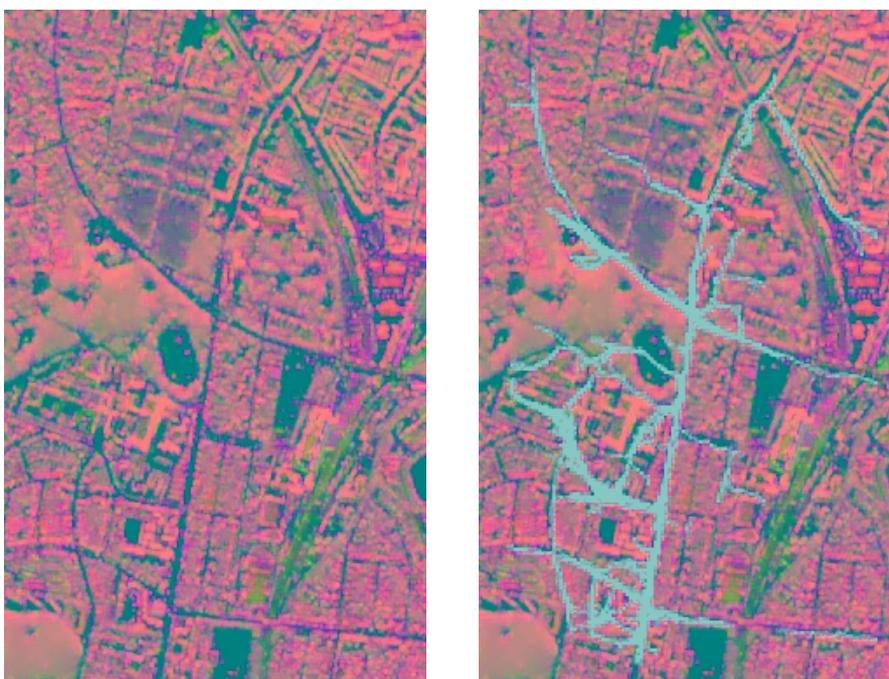
Fig. 4. Speckle reduced EMISAR image, and road detection result using 10 seed points.
