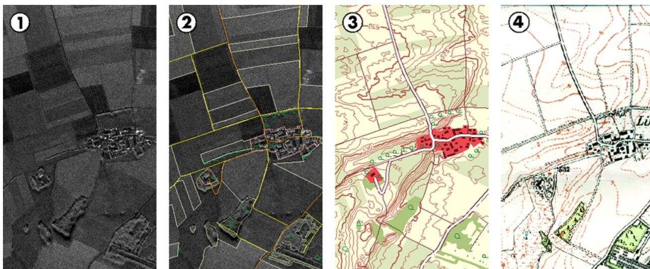
Figure 5: Derivation of a topographic map 1 : 25,000 by visual image interpretation:
