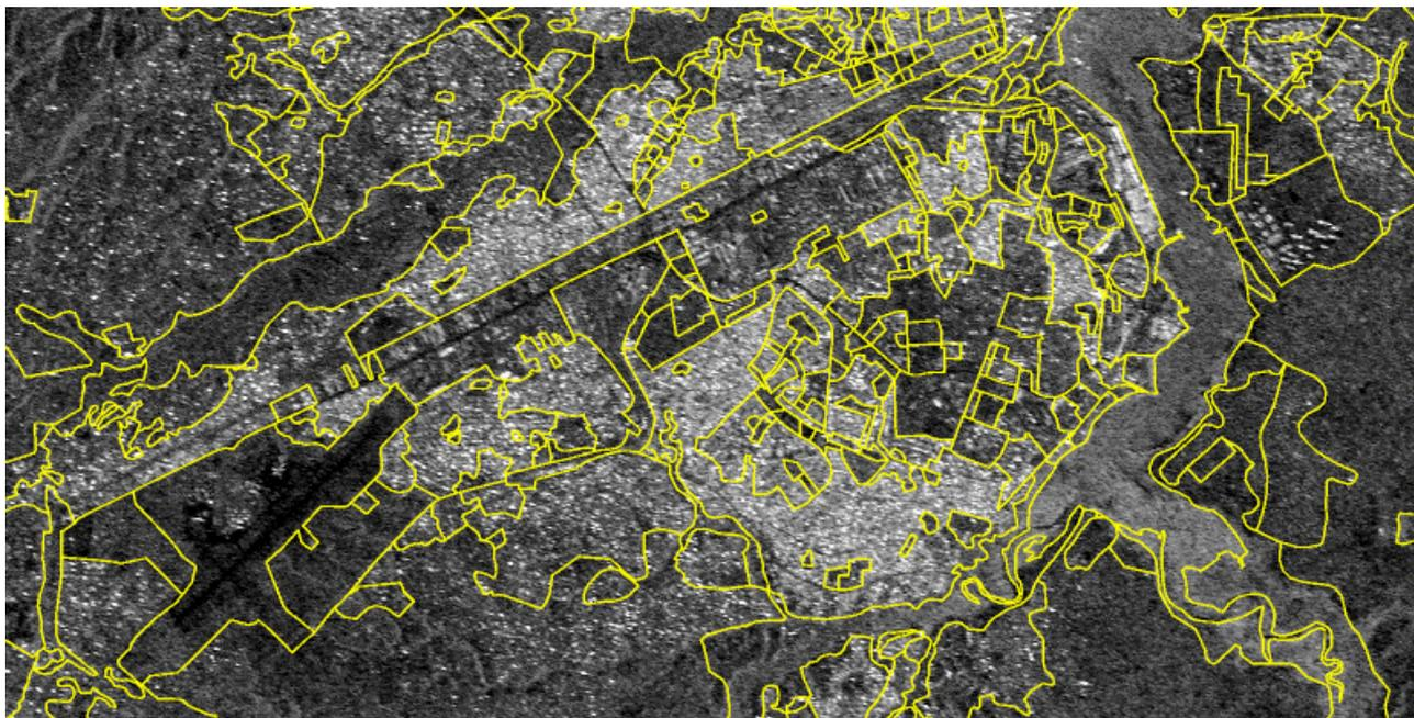
Figure 4. Manual segmentation of land use from vertical aerial photographs of 1992 (1:12,500 and 1:52,000), produced by ITC, The Netherlands, projected on the sum image of the tandem pair of 3-4 October 1997.
