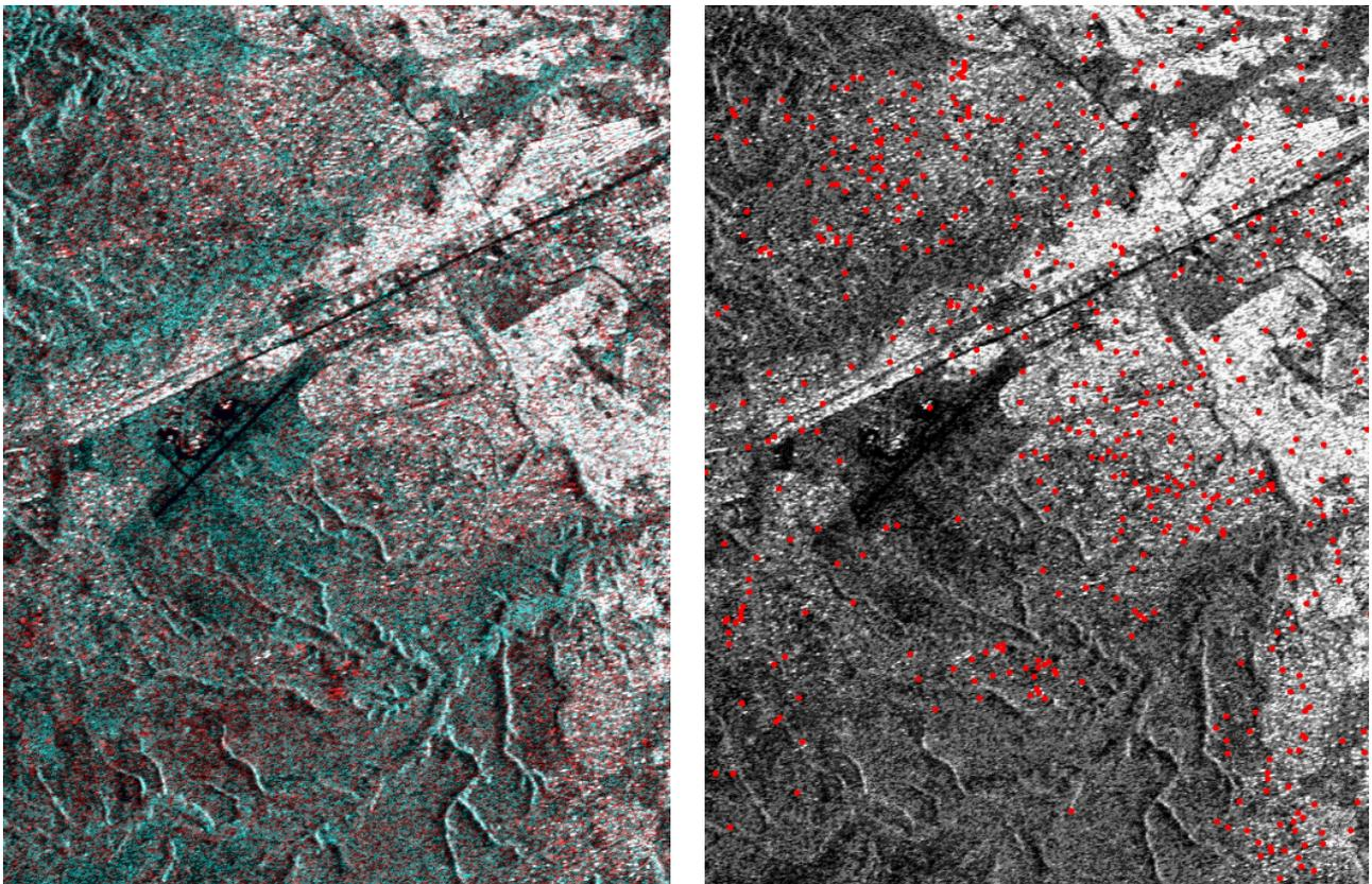
Figure 3. Colour composite of the images of 29 January 1996 (cyan) and 14 December 1998 (red), and the detected new objects projected on the image of 14 December 1998 (right). The less-dense expanding areas show most new objects.
