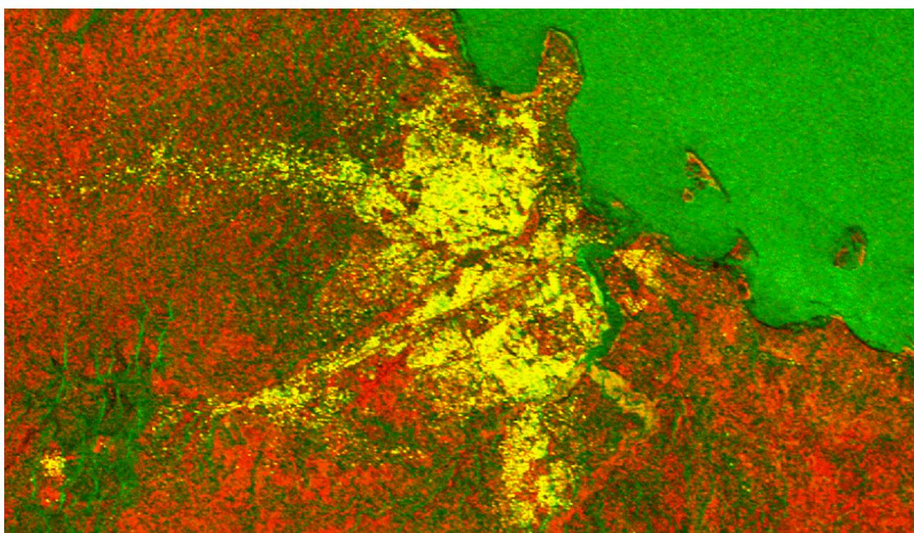
Figure 7. Colour composite of the coherence image (red) and the intensity sum image (green) of tandem pair 32516-12843. Urban objects have both a high intensity and coherence and will therefore be yellow. Forest has medium intensity and low coherence and will therefore be green (e.g. the Pugu Forest Reserve, bottom left).
