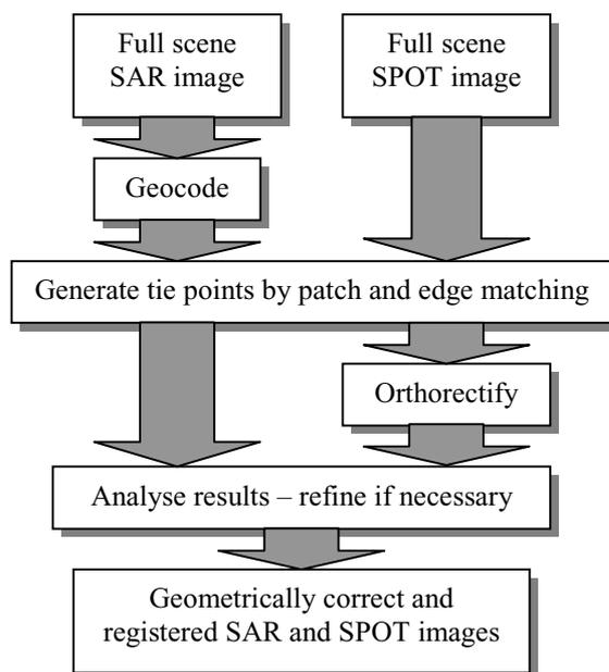
Figure 6. Automatic orthorectification of SPOT imagery
