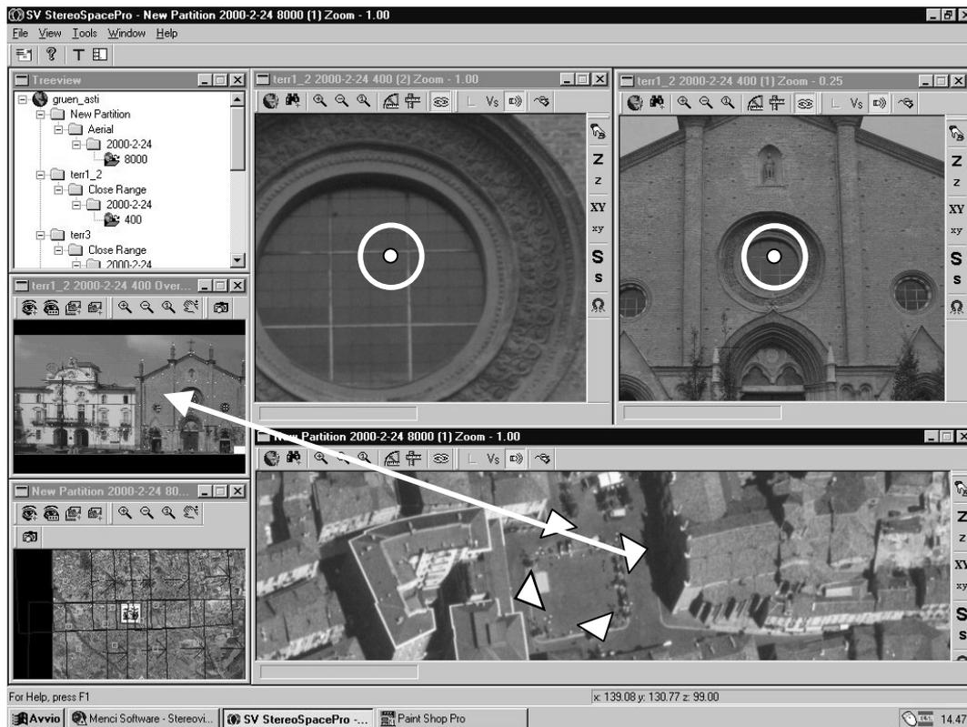
Figure 7. Hot-spots joining aerial and terrestrial blocks
