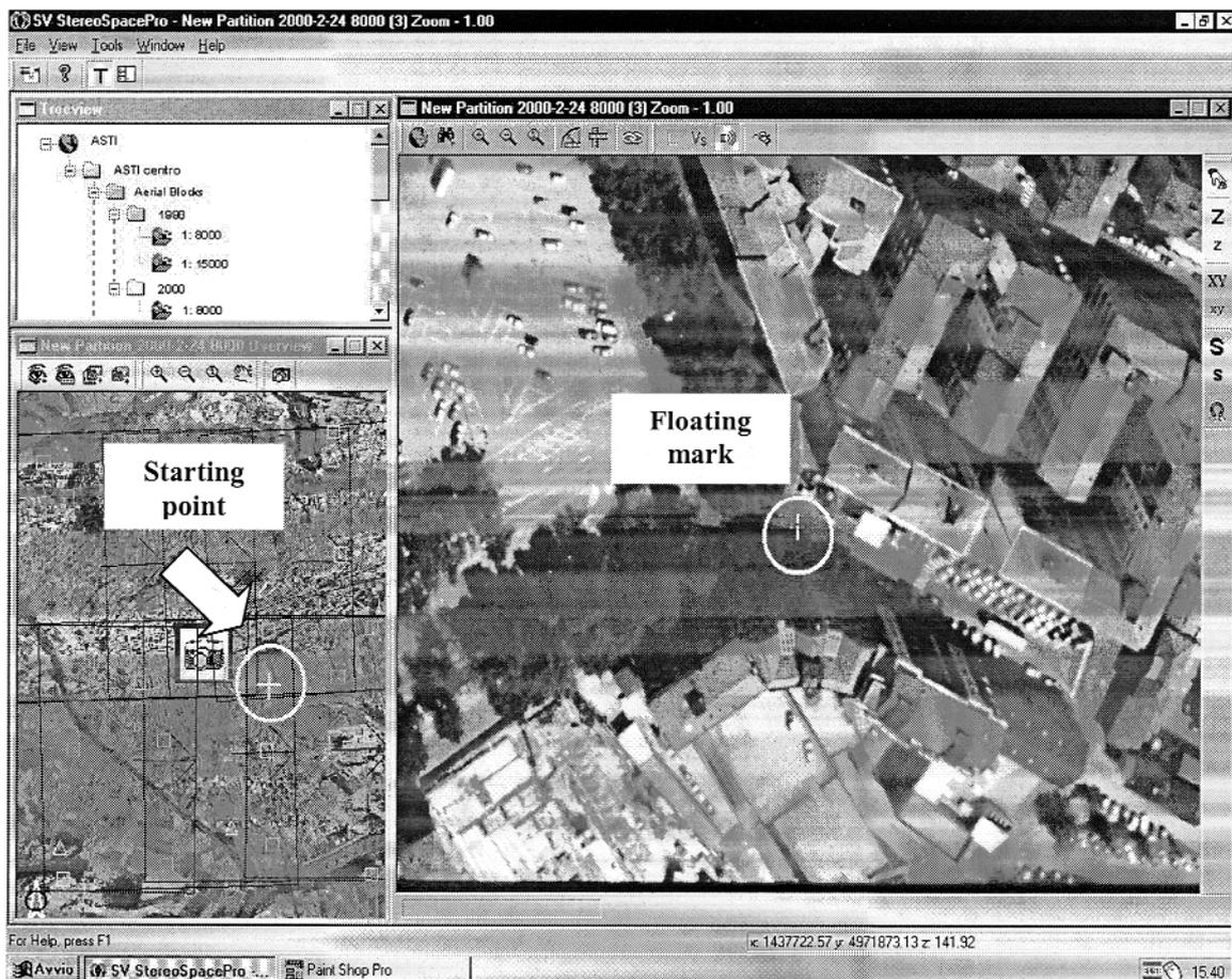
Figure 3. Starting the 3D NAVIGATOR
