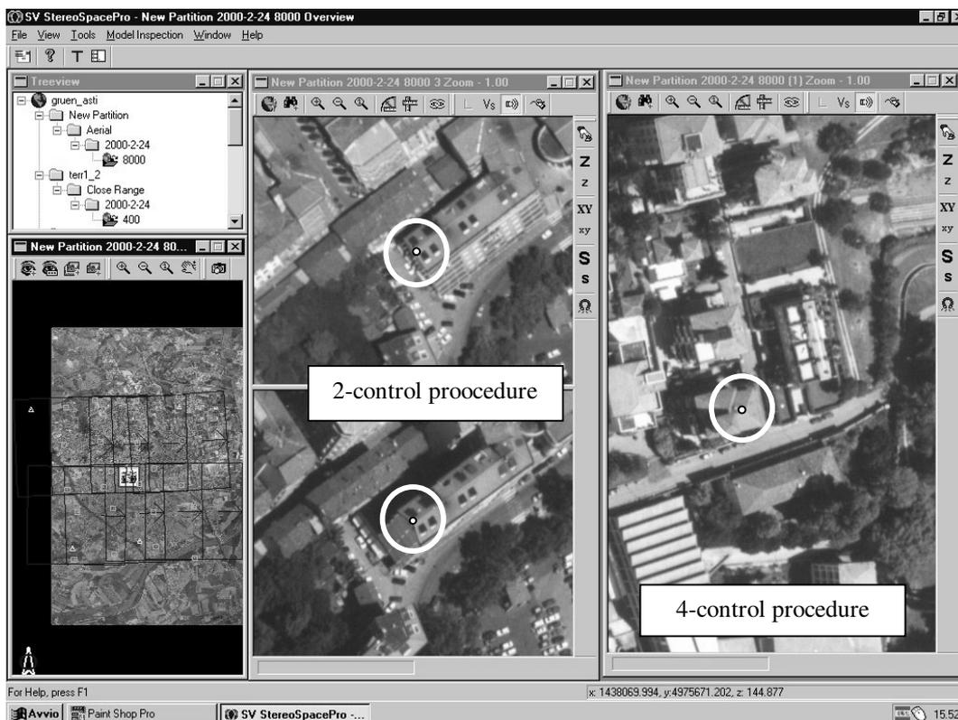
Figure 8. Stereoscopic collimation of single points in an aerial block
