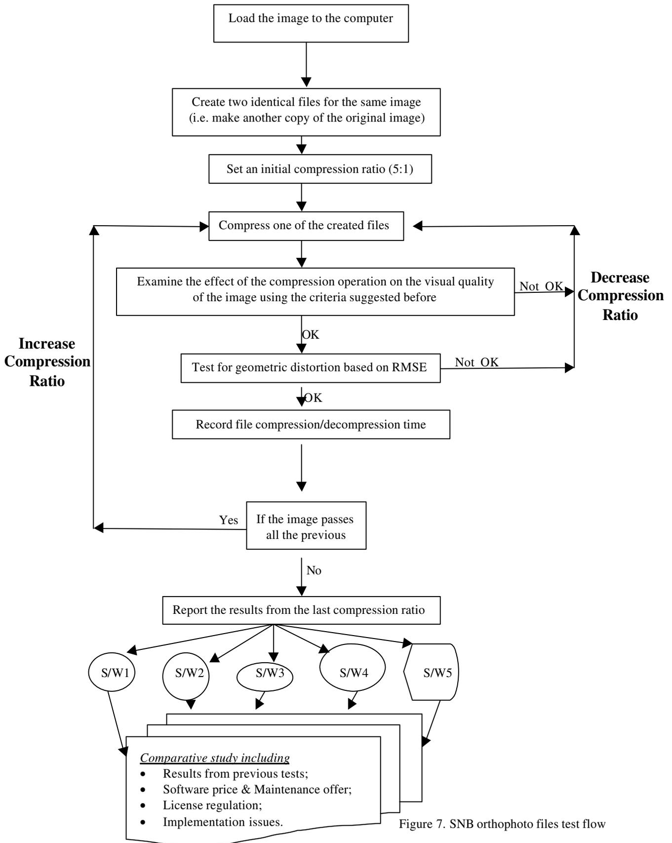
Figure 7. SNB orthophoto files test flow
