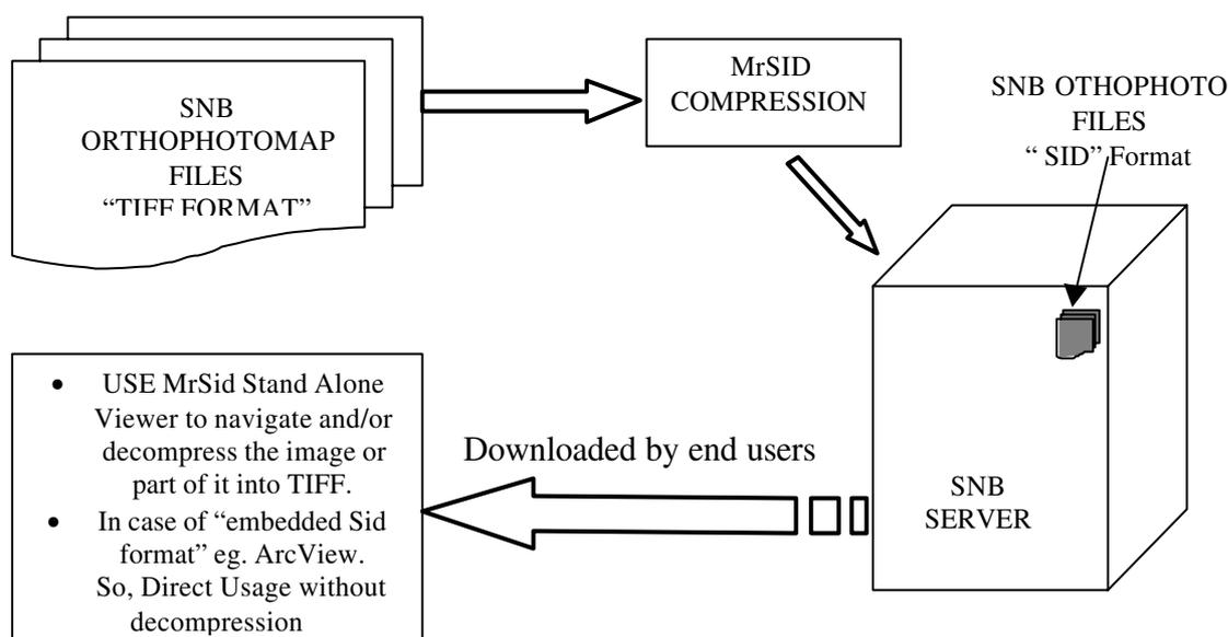
Figure 18. SNB orthophotomap database work cycle
