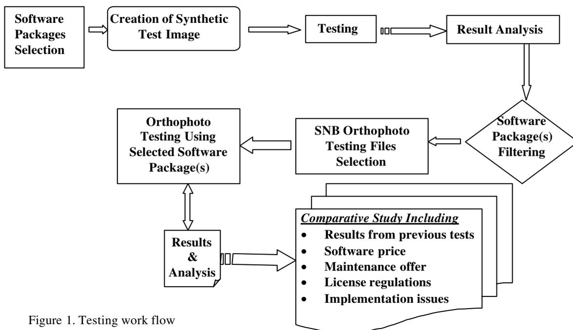
Figure 1. Testing work flow
