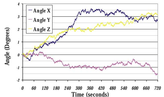
**Figure 1: Angular Drift from Low-cost Strapdown IMU (Crossbow DMU-FOG)**
