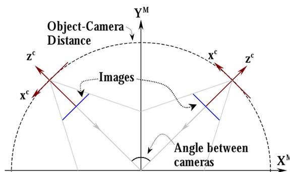
Figure 4: Imaging Geometry for Simulations
